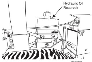
Figure 7-2. Hydraulic Oil Reservoir
